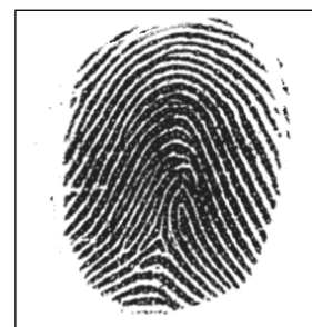
Good image: fingerprint in the middle, medium pressure to the sensor.
