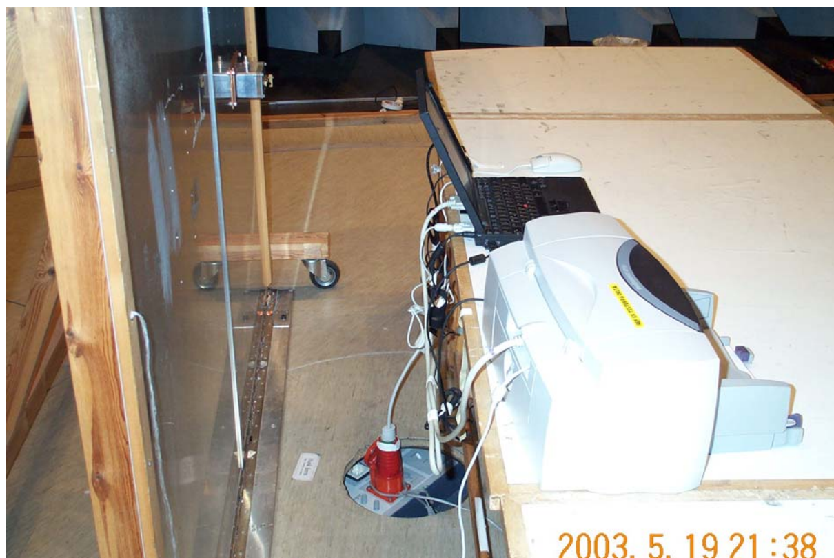
Photo A2.3 AC mains conducted emission measurement.
