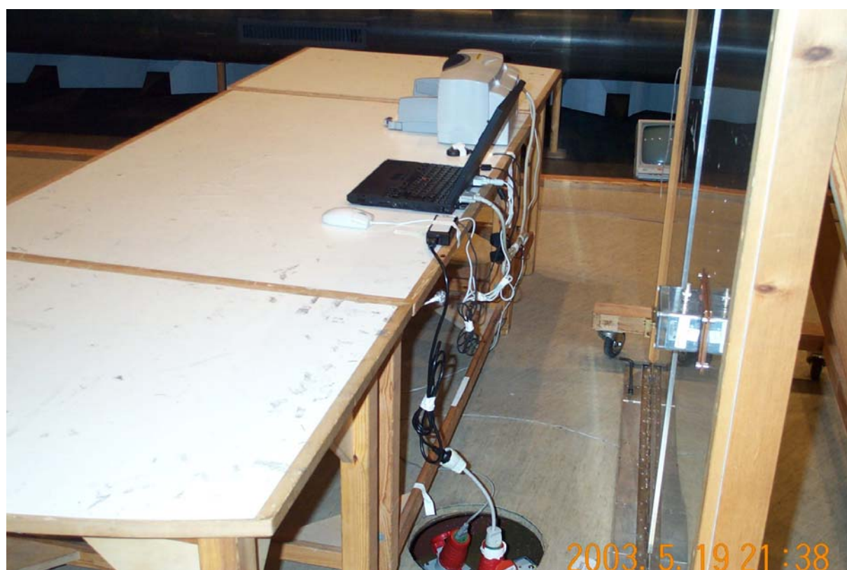
Photo A2.2 AC mains conducted emission measurement.
