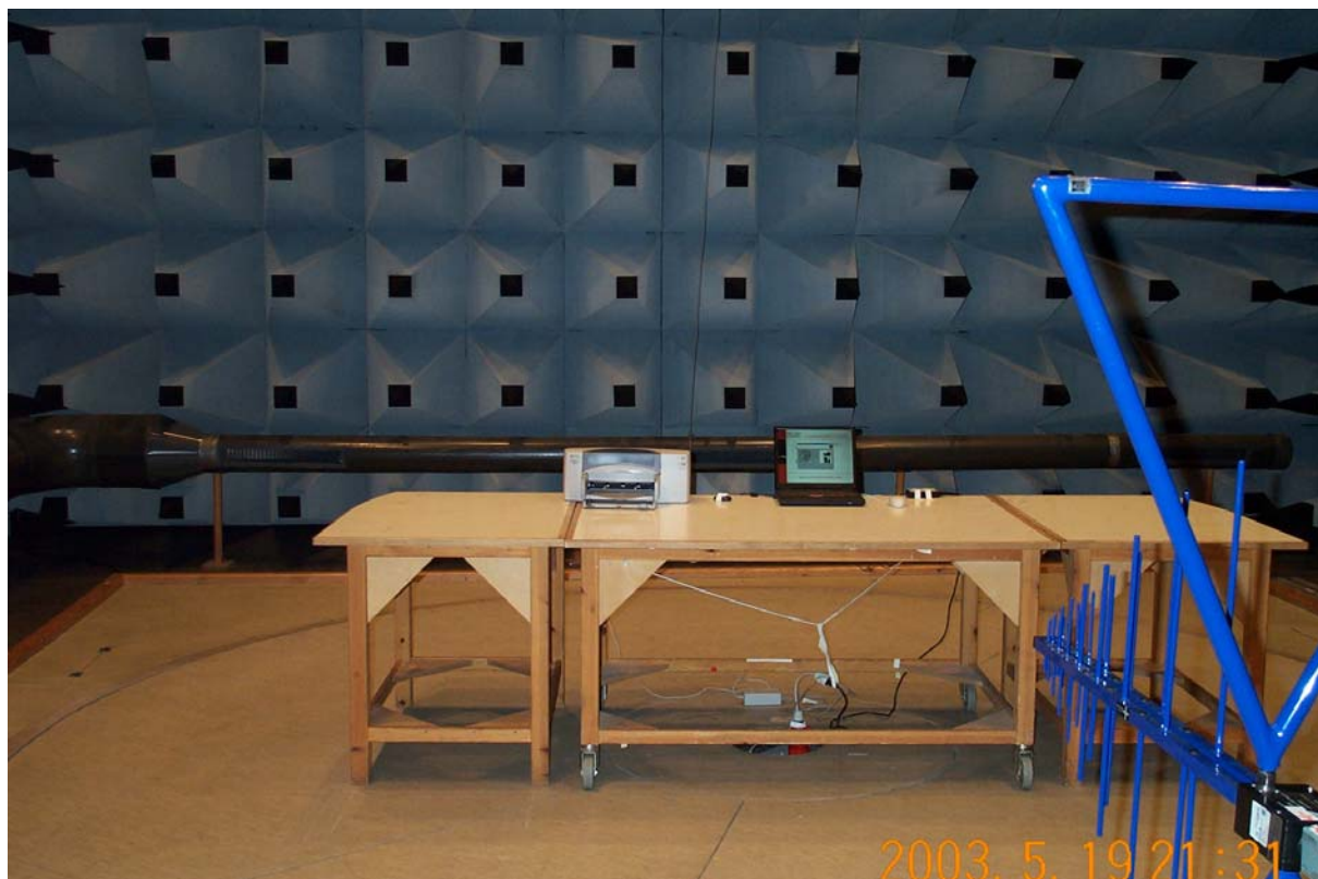
Photo A3.1 Radiated electromagnetic field measurement.
