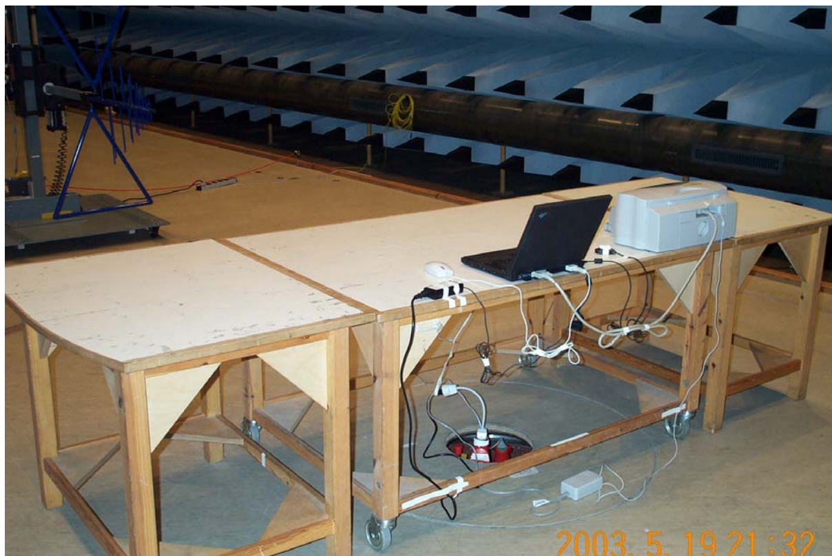
Photo A3.2 Radiated electromagnetic field measurement.
