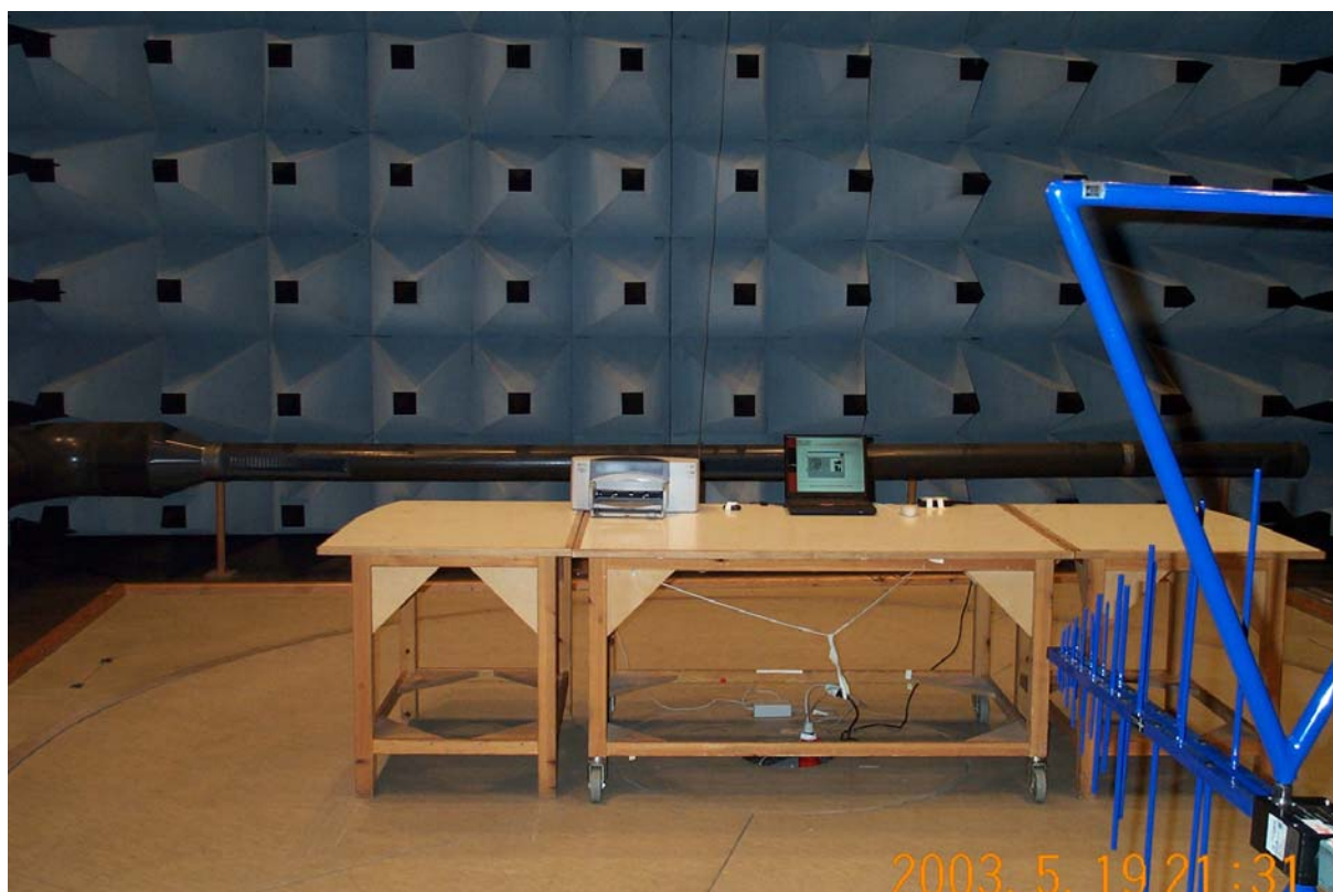
Photo A3.1 Radiated electromagnetic field measurement.
