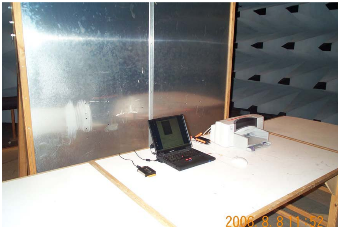
Photo 4.1.1 Test setup regarding measurement of RF voltage on AC mains.
