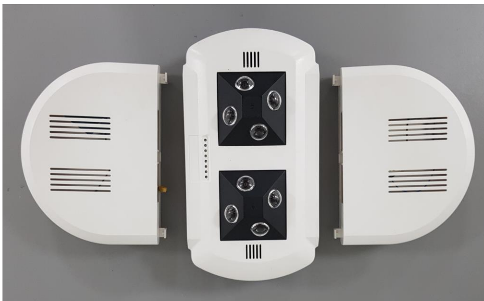
Photo 3: EUT with Antennas Removed
