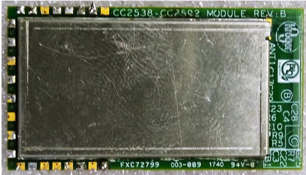
Photo 1: RF Module Front view
