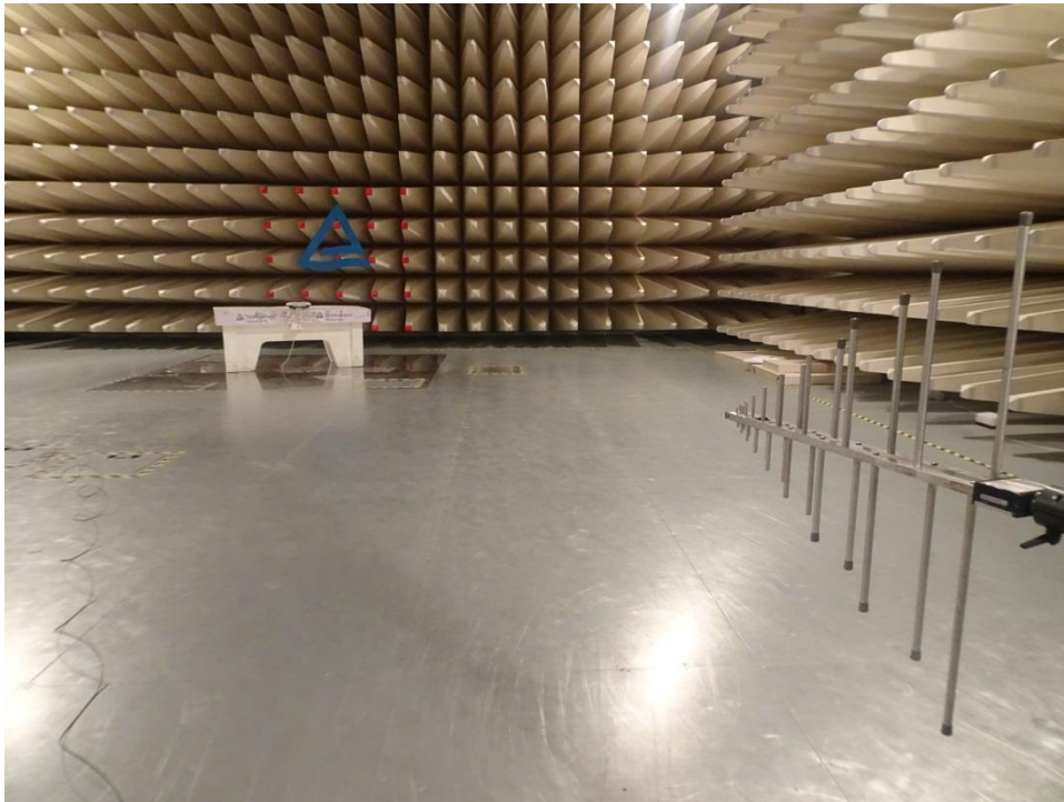
Photo 5: Log periodic antenna Vertical polarization
