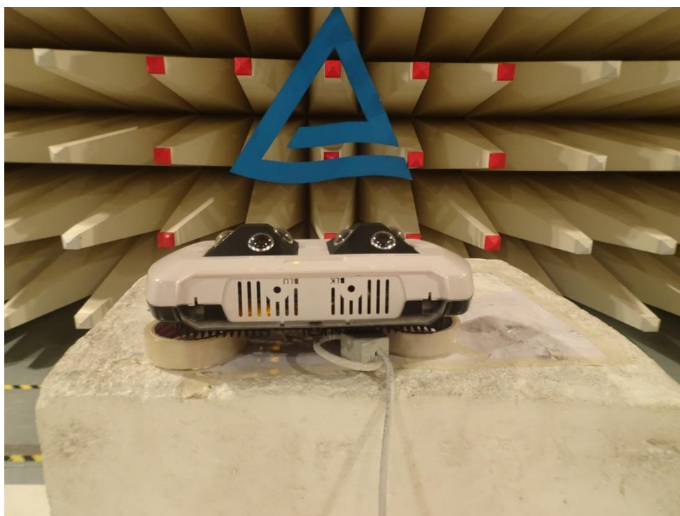
Photo 12: EUT setup for above 1GHz
