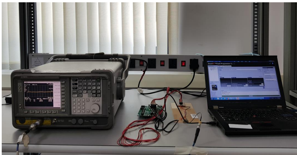
Photo 13: Antenna Port measurement
