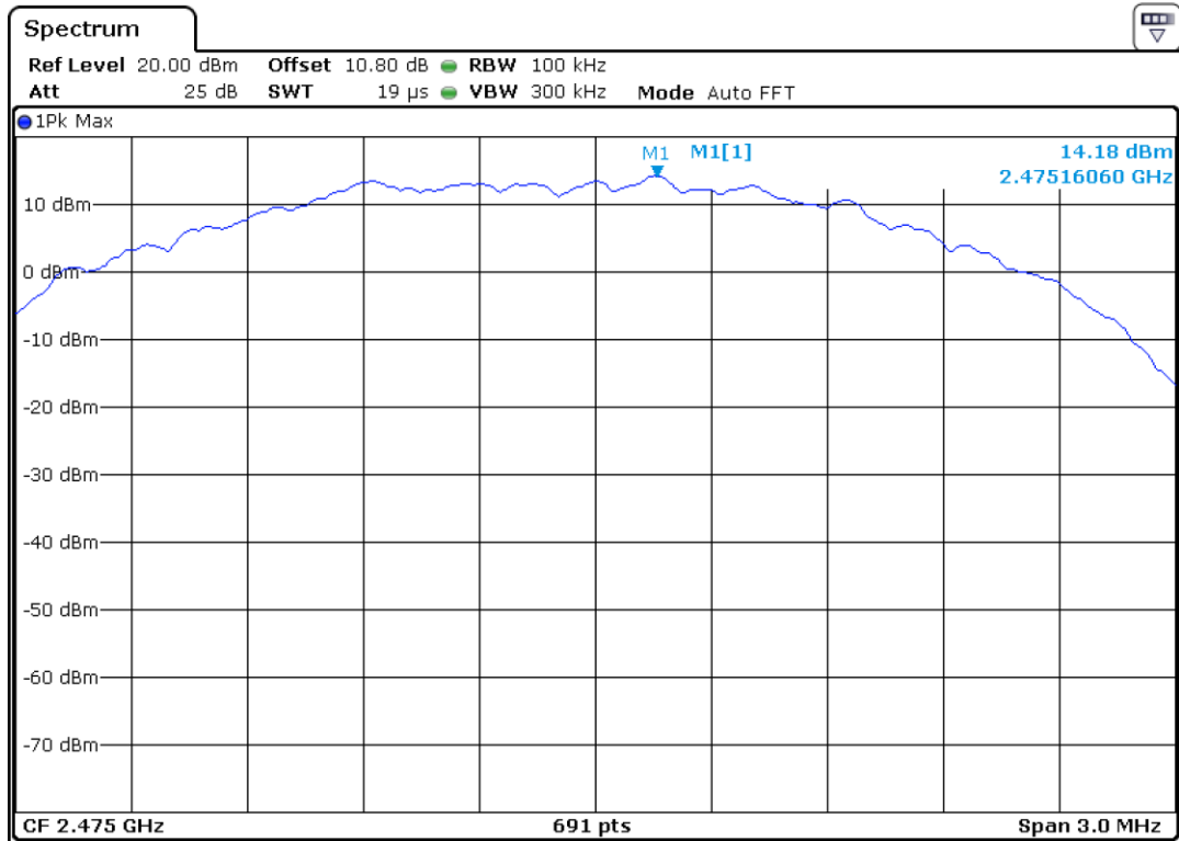
Reference Level Plot - Channel no. 25- 2475 MHz
