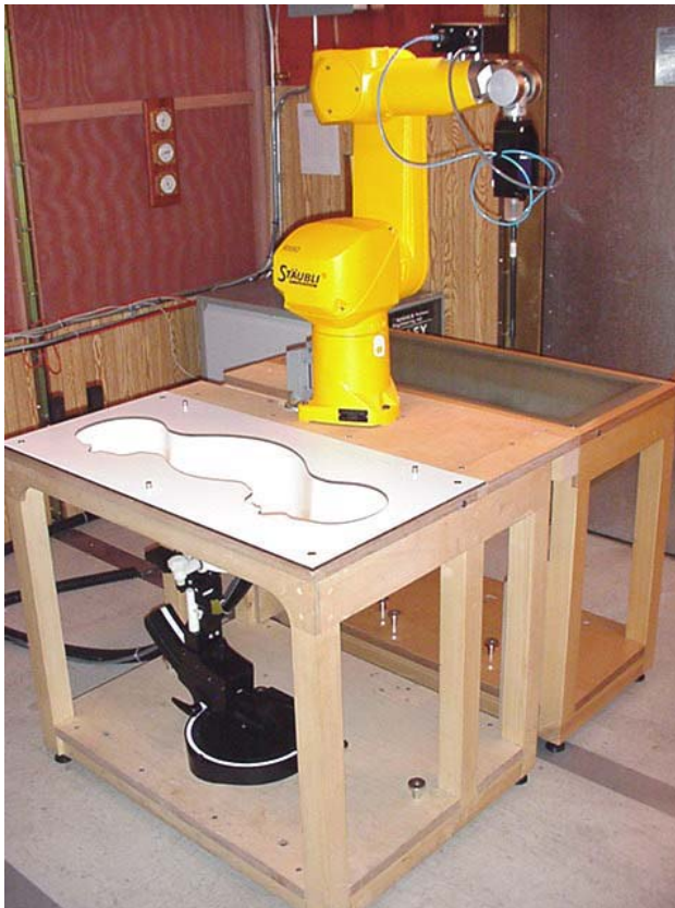
DASY4 Measurement System with SAM Phantom
