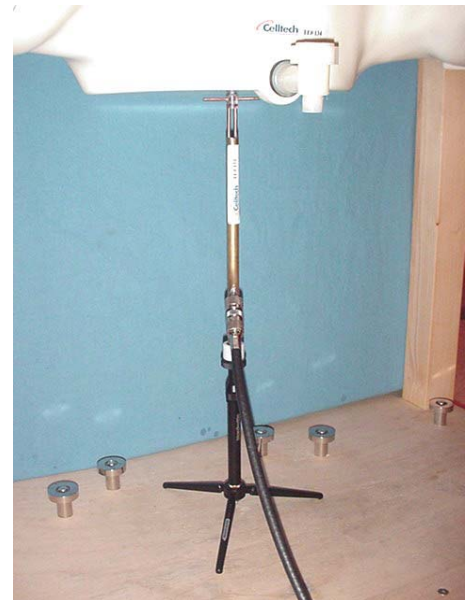
1900MHz Dipole Setup
