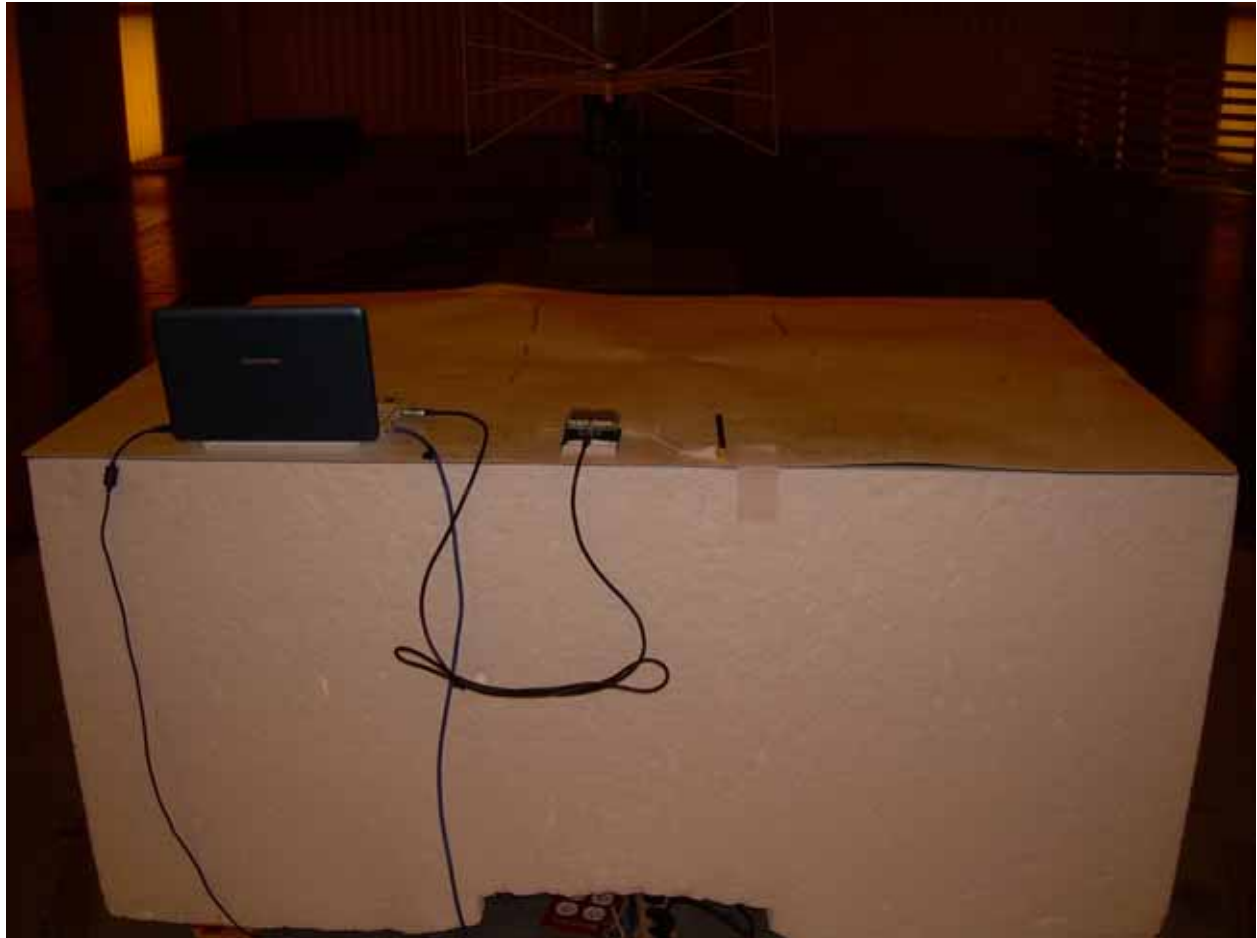
Photograph 2 – Back View Radiated Emission – Horizontal EUT Configuration
