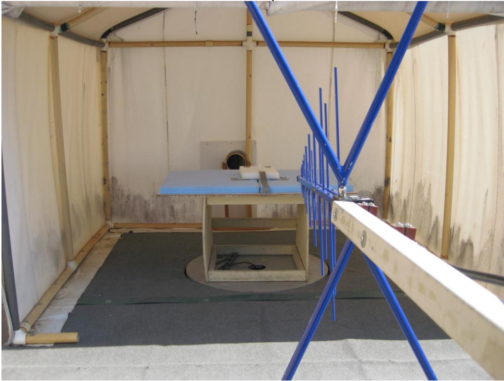
Radiated Test Set-up below 1 GHz
