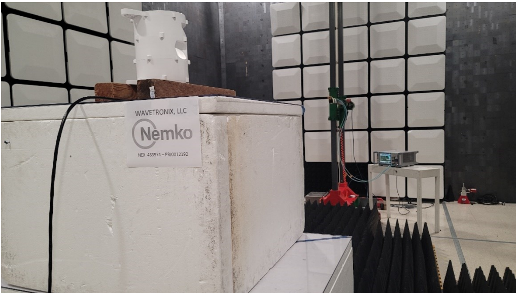
Figure 23 – Occupied bandwidth test, rear view
