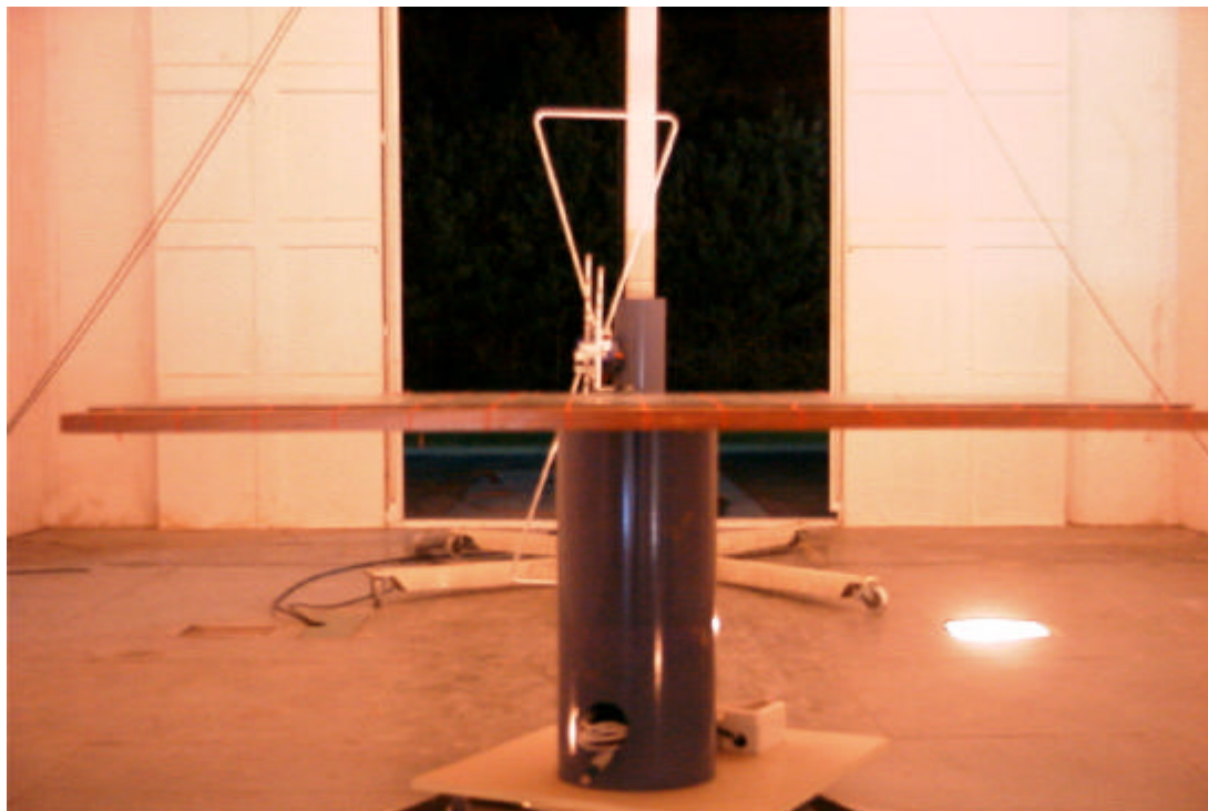
Figure 4(b) : Radiated Emission 30MHz ~ 1000MHz
