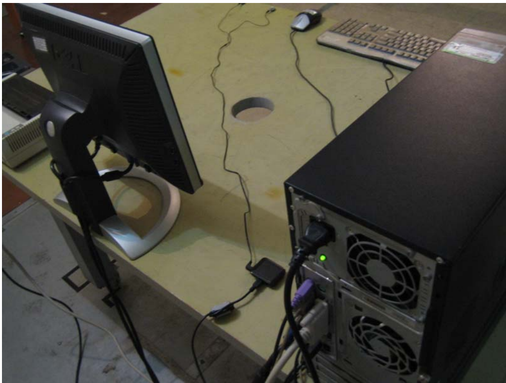
Conducted Emissions (PC power line) - Rear View
