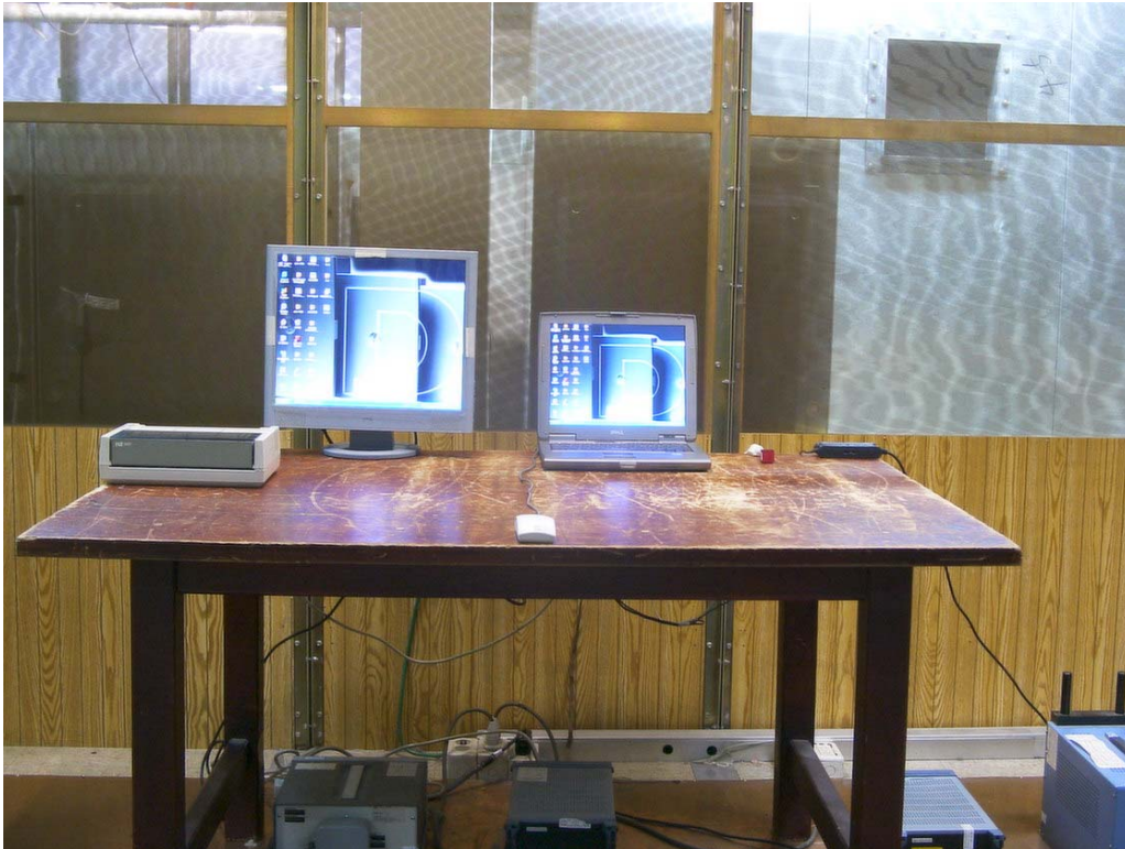
Conducted Emissions (File up/download mode) - Front View
