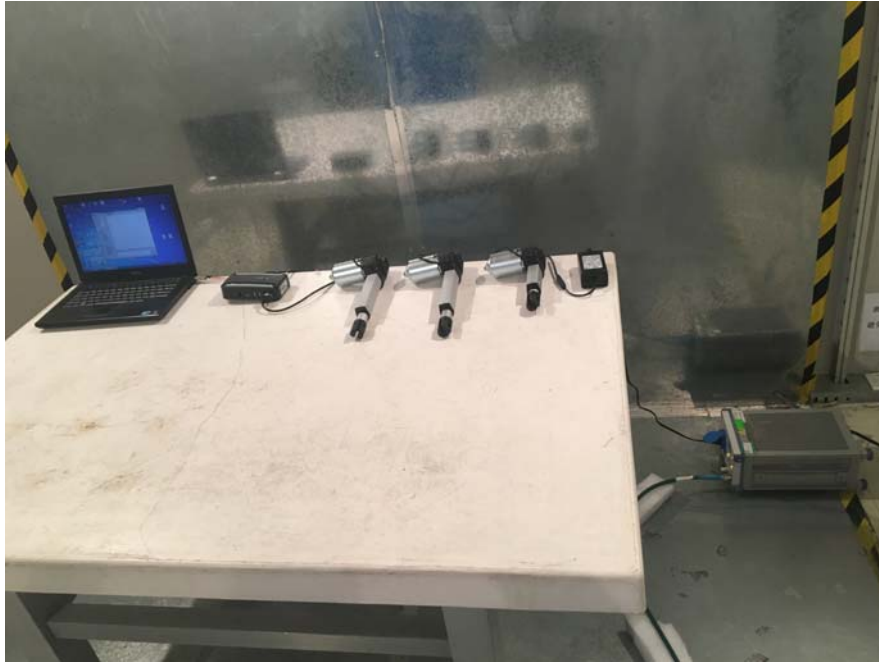
Conducted Emissions (Side View)
