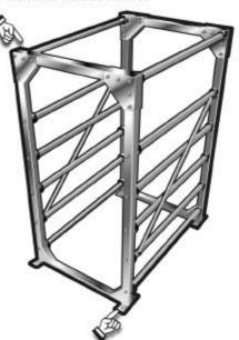
Fix the antenna using 1/ainch (12mm) bolts through the holes in the feet.
