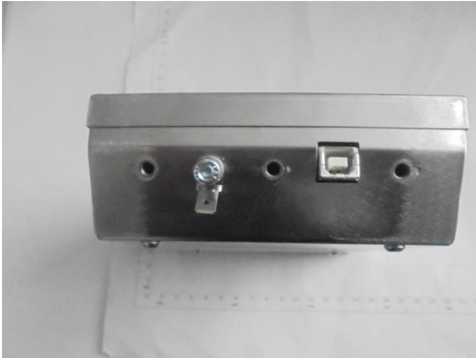
Photograph 3: Power cable connector
