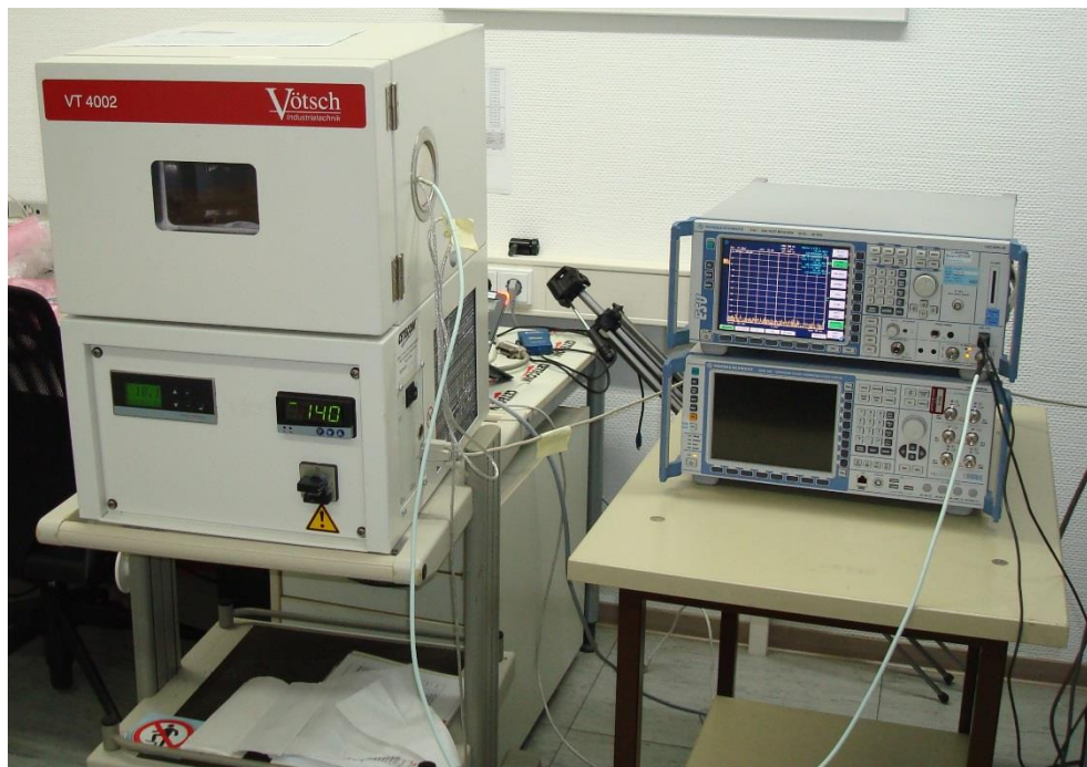
Photograph 3: EUT Test setup within temperature chamber
