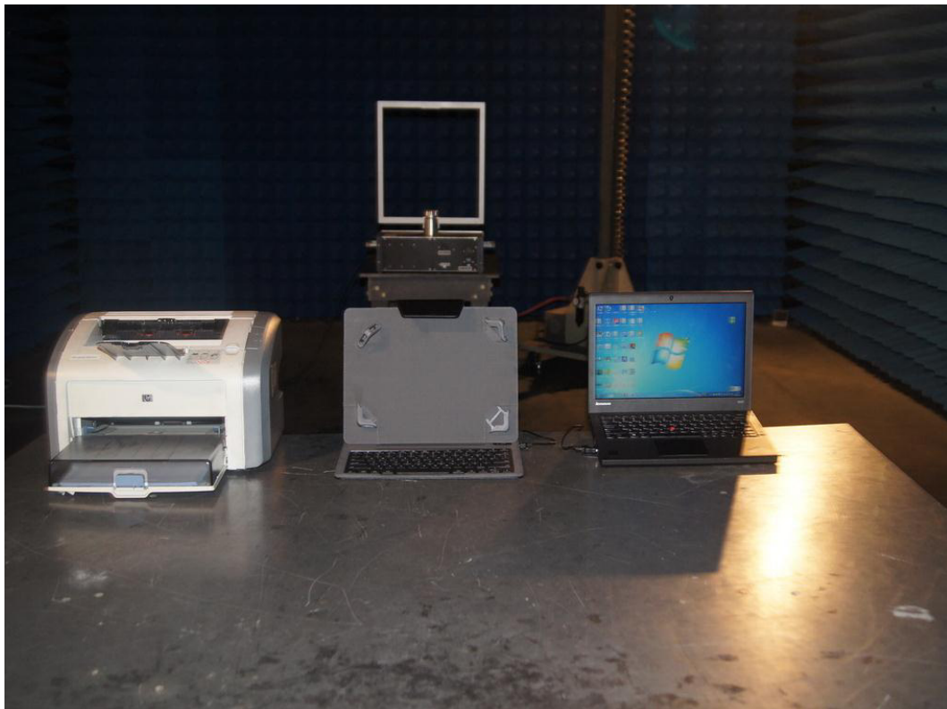
Photograph 6: Set-up for Radiated Emissions, 9 KHz-30MHz
