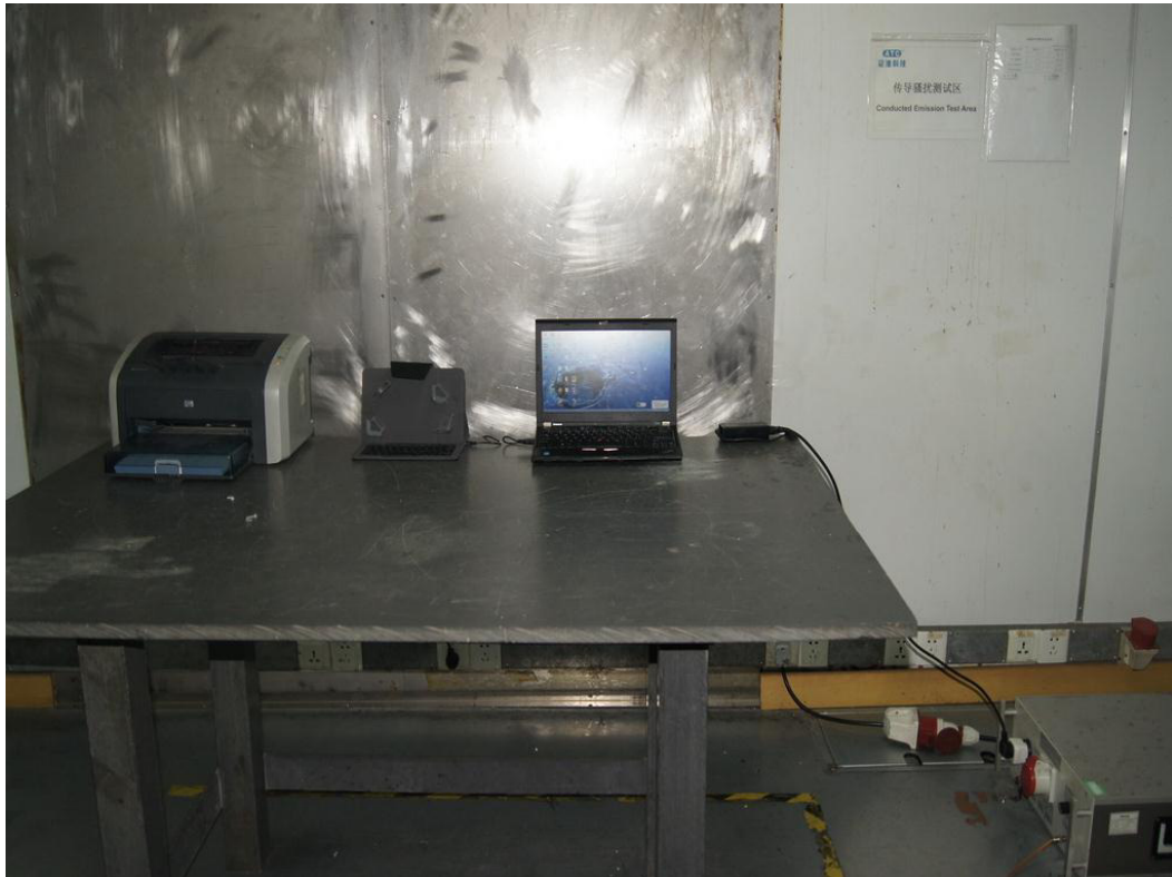
Photograph 6: Set-up for Radiated Emissions, 9 KHz-30MHz
