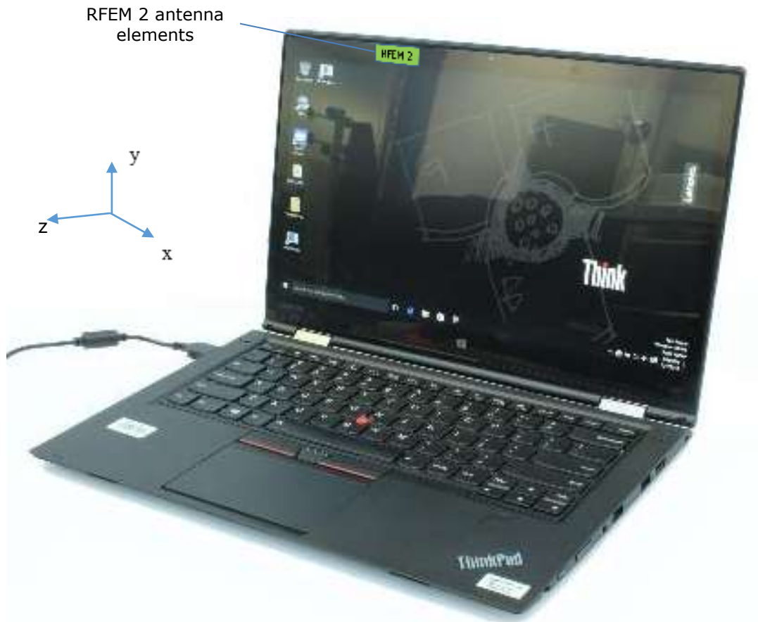
Figure 7 – Active antenna inside the platform
