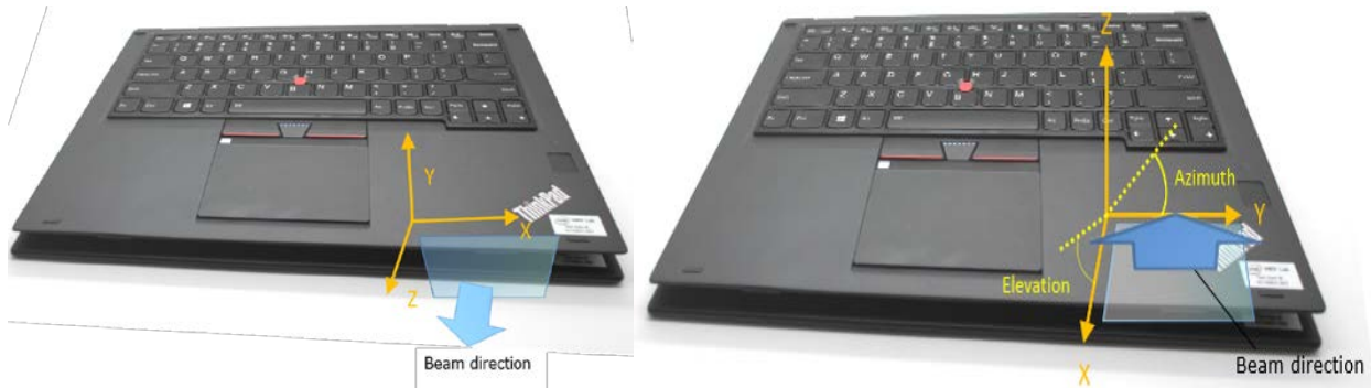
Figure 3 – Search Planes are the x-y planes (i.e. the transparent plane as illustrated in this picture- Left: Edge plane Right: Base plane)
