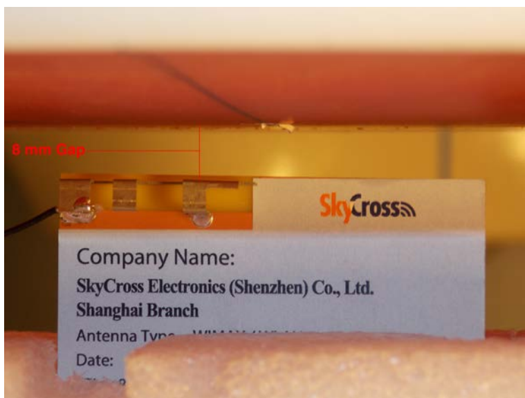
Test Position Side D 8 mm Gap
