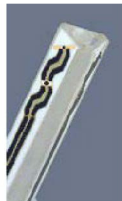
Figure 2.3 Probe Thick-Film Technique
