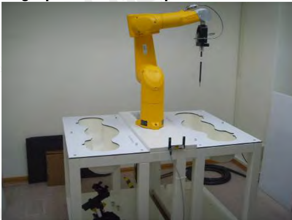
Fig.1 Photograph of the SAR measurement System
