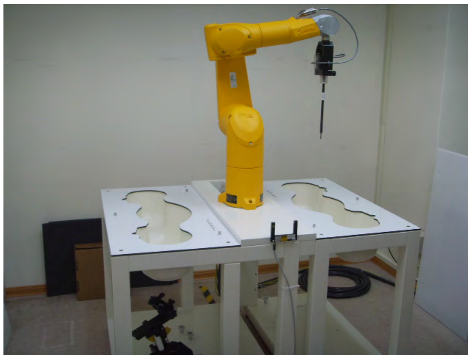
Fig.1 Photograph of the SAR measurement system
