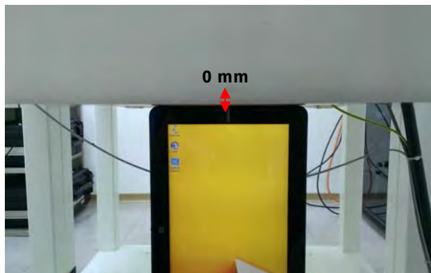
Fig.5 EUT left side to flat phantom
