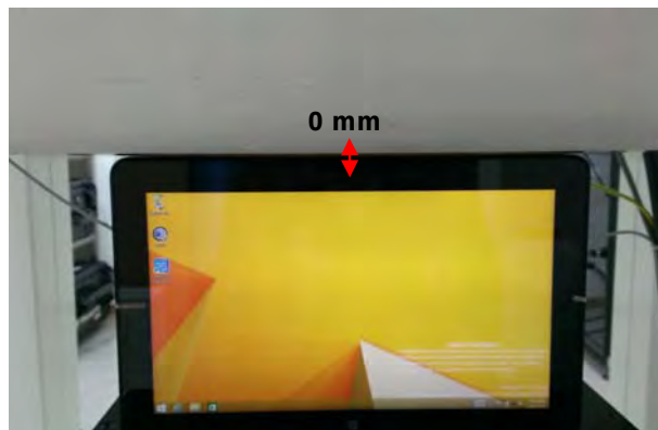
Fig.4 EUT top side to flat phantom
