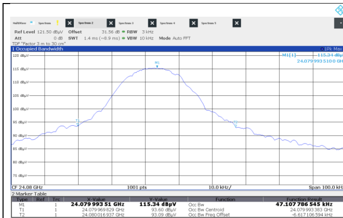
Figure 7.6-3: 99% occupied bandwidth, sample plot Low Ch
