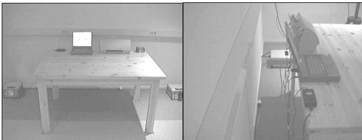
Picture 1. AC conducted emission measurement setup.
