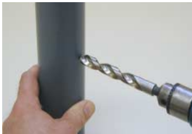
Figure 2-7. Drilling Pool Pipe
