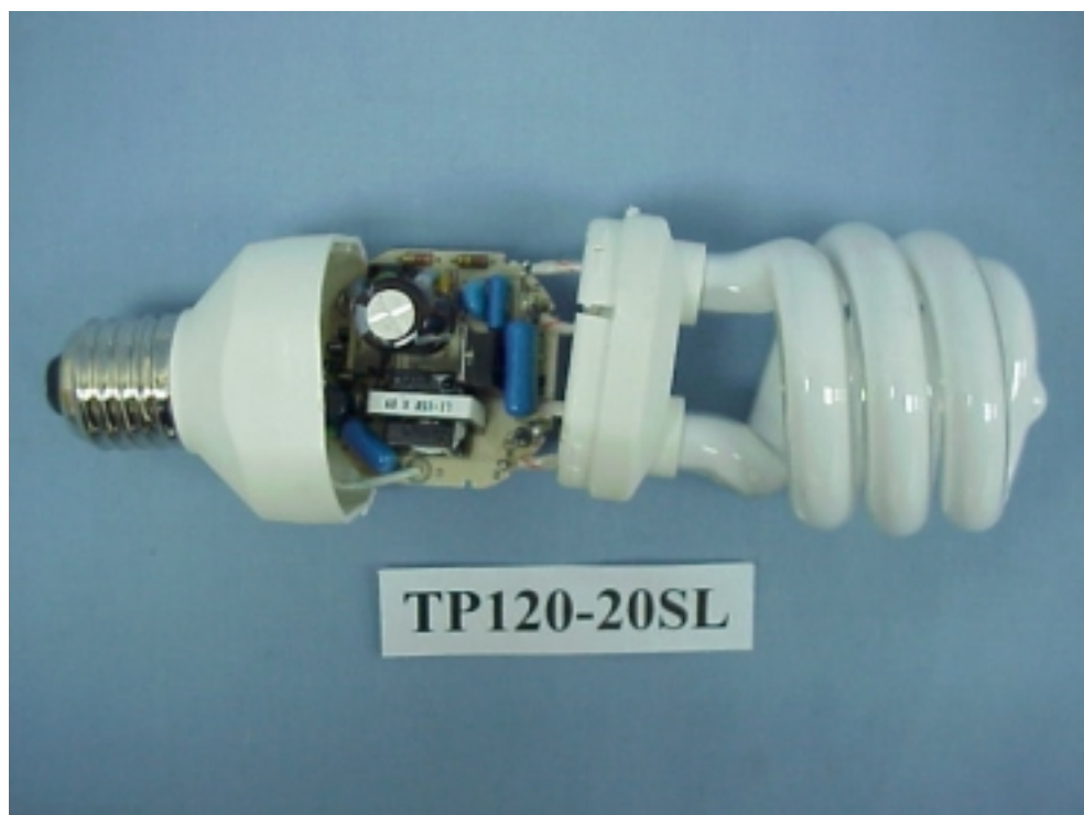
Figure 10 Compact Fluorescent Lamp (M/N: TP120-20SL) Cover Removed
