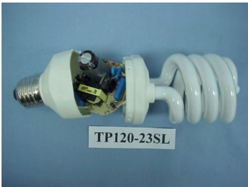
Figure 12 Compact Fluorescent Lamp (M/N: TP120-23SL) Cover Removed
