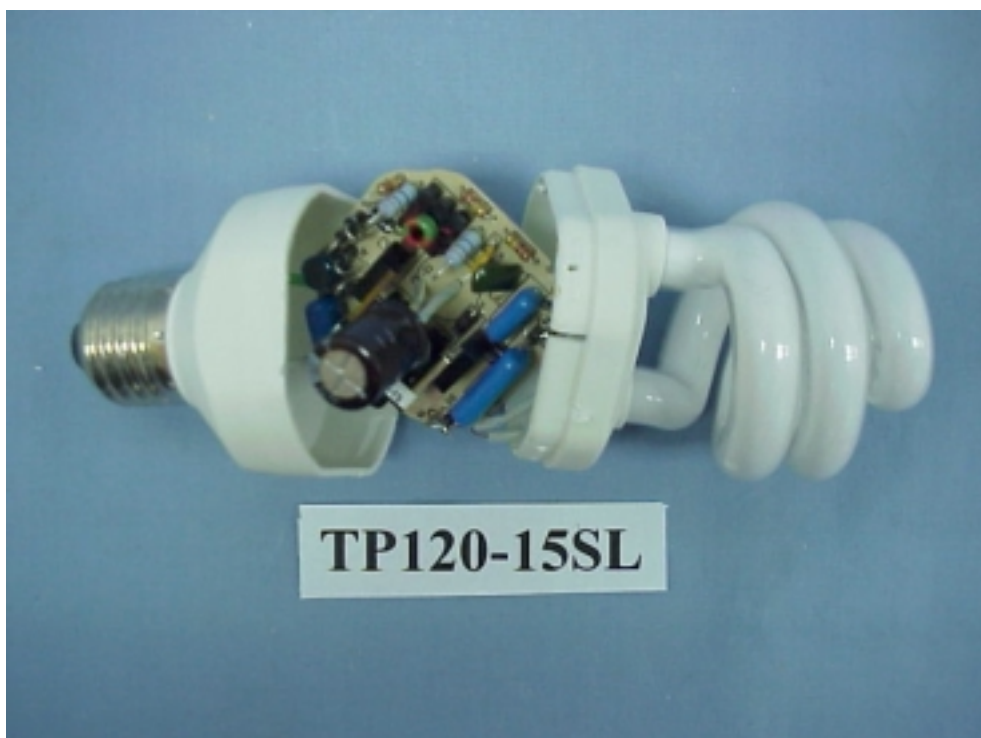
Figure 8 Compact Fluorescent Lamp (M/N: TP120-15SL) Cover Removed
