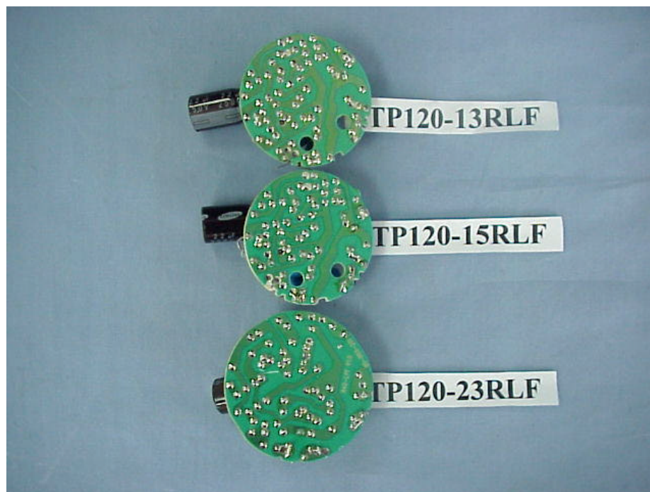
Figure 3. Compact Fluorescent Lamp (M/N: TP120-RLF Series) Main Board (Soldered Side)
