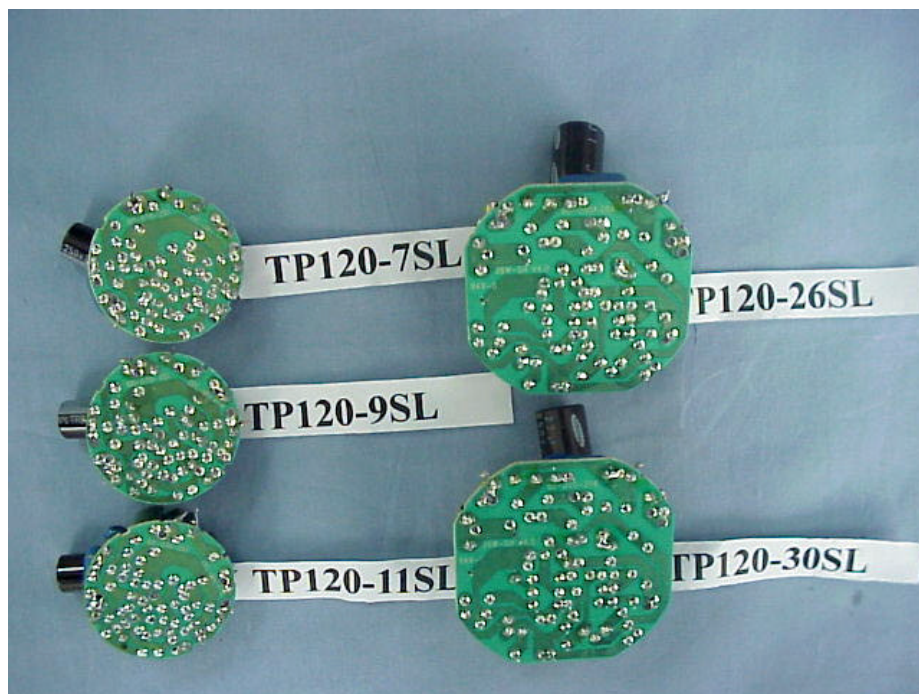
Figure 9. Compact Fluorescent Lamp (M/N: TP120-SL Series) Main Board (Soldered Side)
