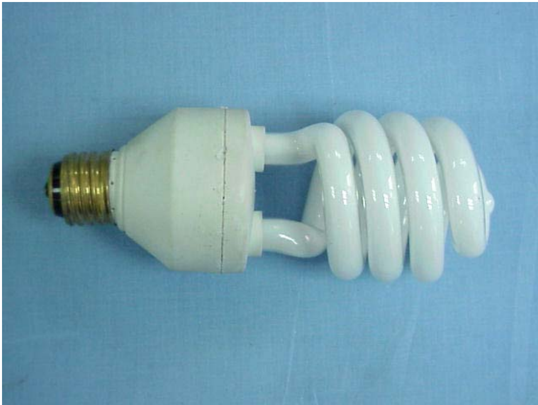
FIGURE 1 COMPACT FLUORESCENT LAMP (M/N: TP 120-25/20/13) GENERAL APPEARANCE
