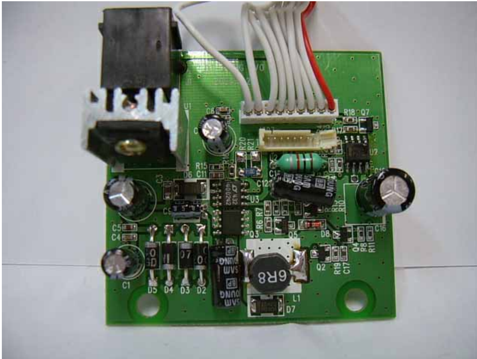
charger pcb top (640x480x16M jpeg)
