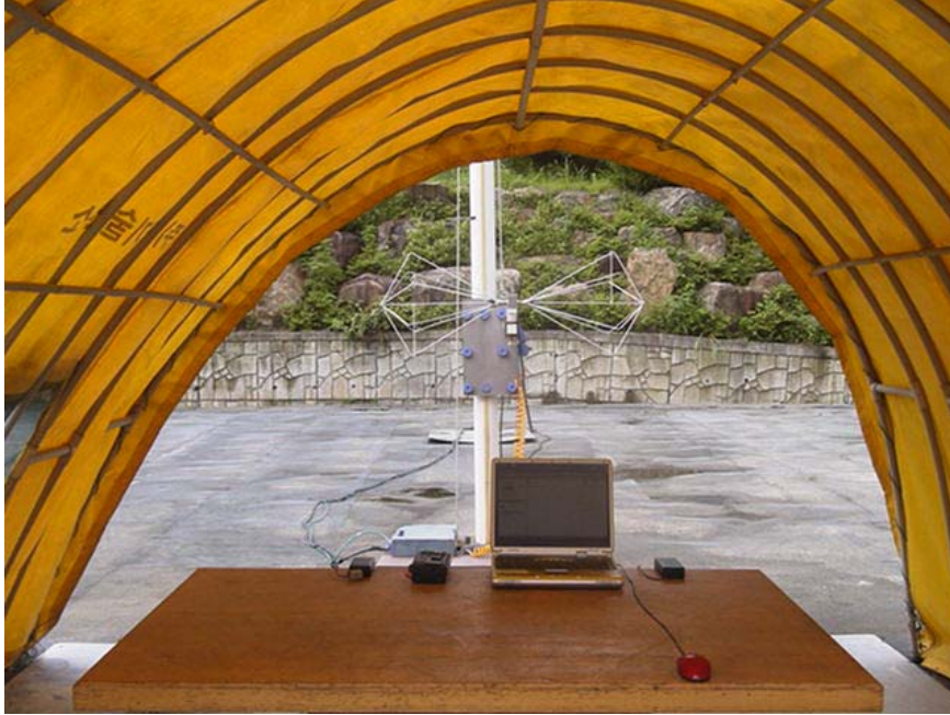
Photograph 1 : Setup for radiated Emissions
