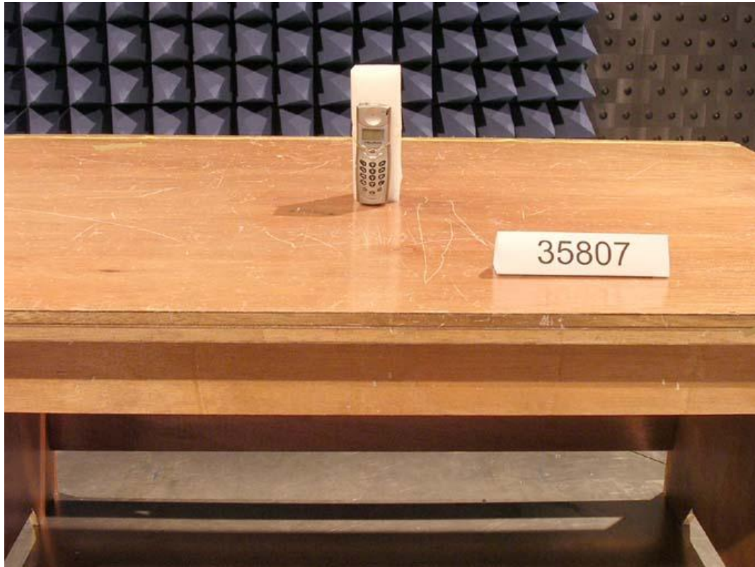
Photo 4: Radiated Emission Test Set-up (Handset)
