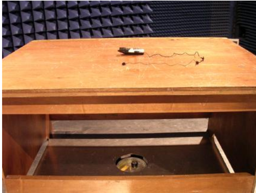
Photo 2: Radiated Emission Test Set-up (Handset)
