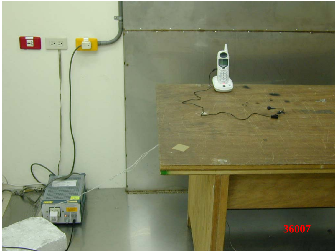
Photo 1: Conducted Emission Test Set-up photo
