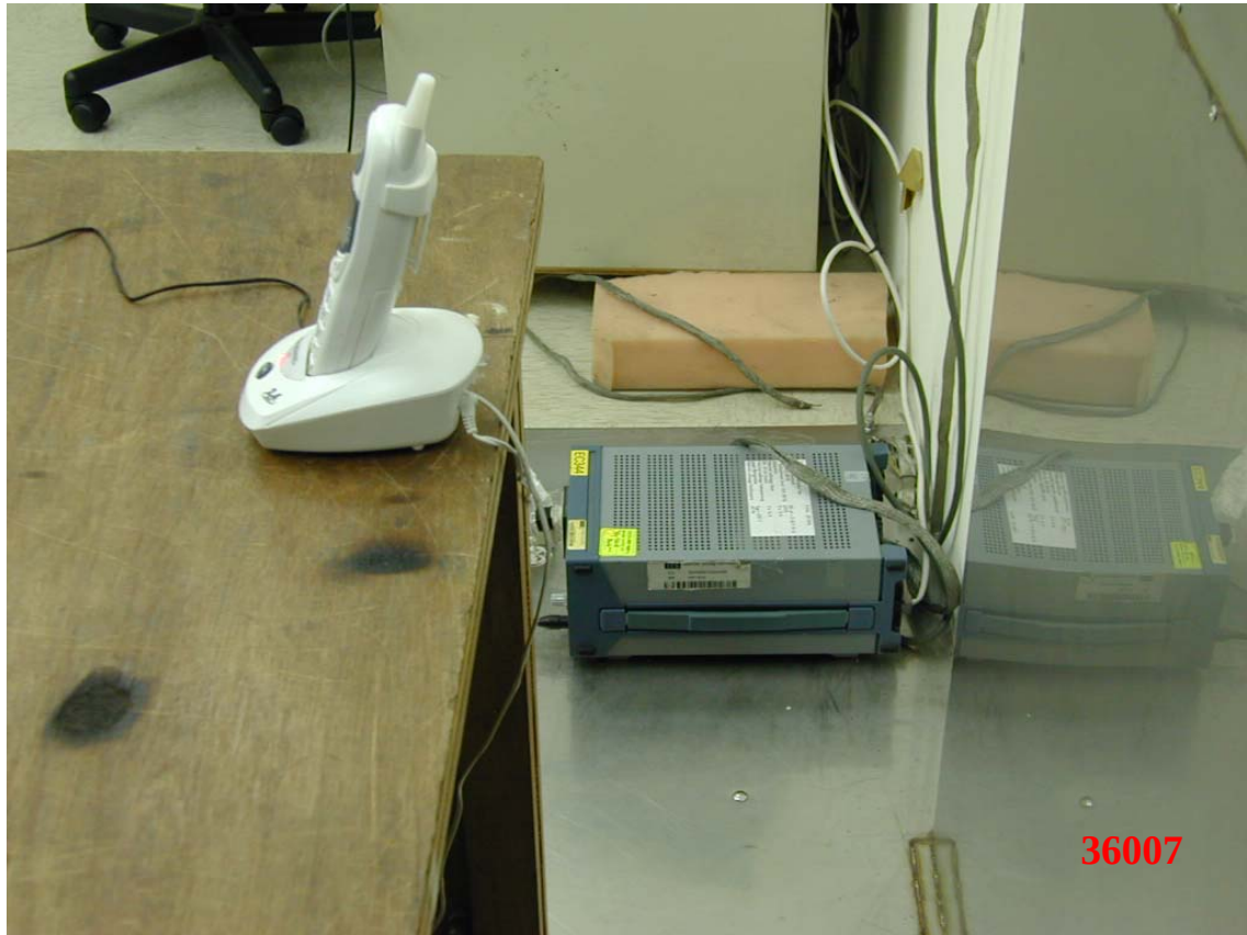
Photo 2: Conducted Emission Test Set-up photo
