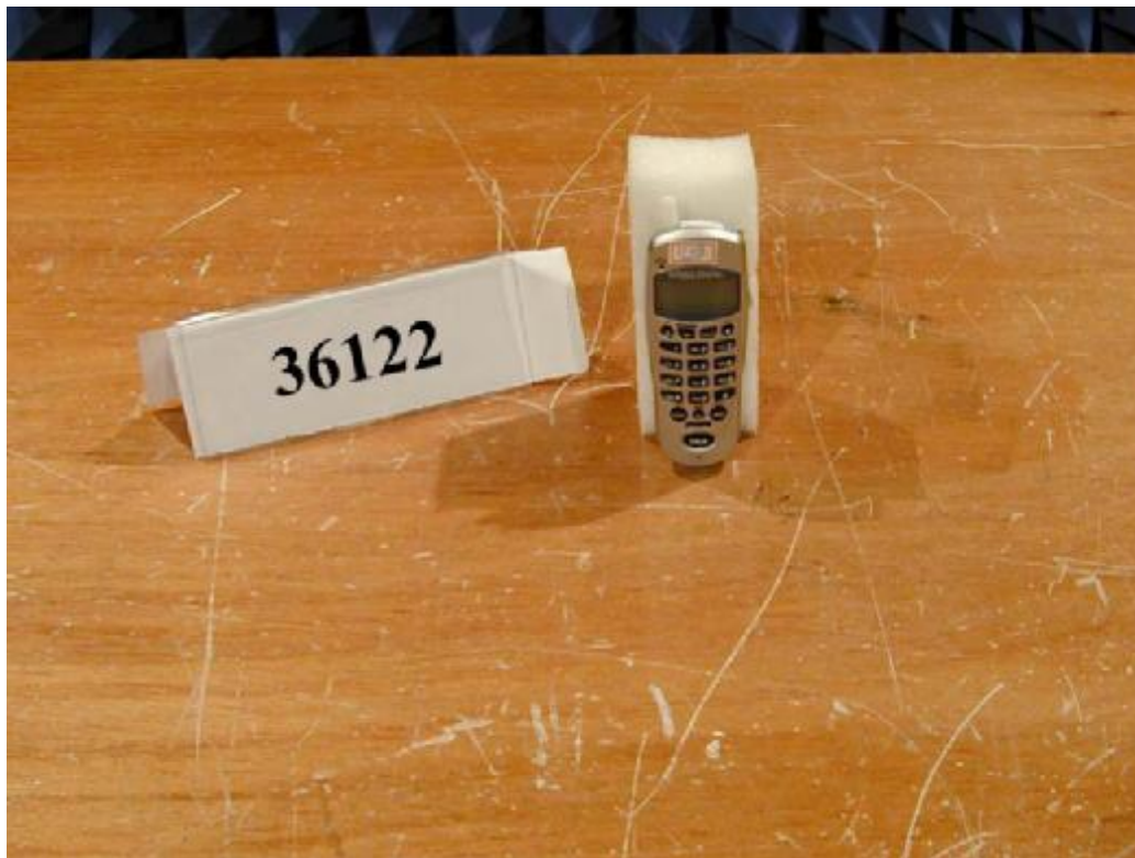
Photo 7: Radiated Emission Test Set-up (Handset)
