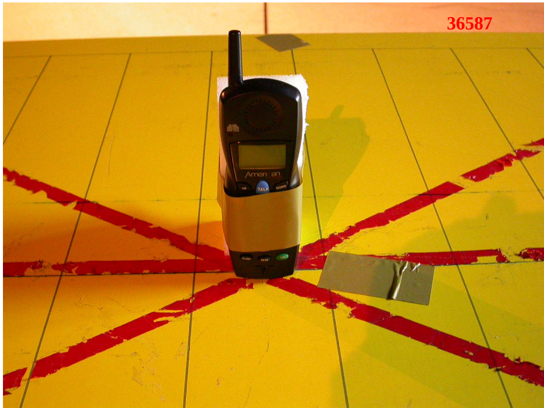
Photo 4: Radiated Emission Test Set-up photo
