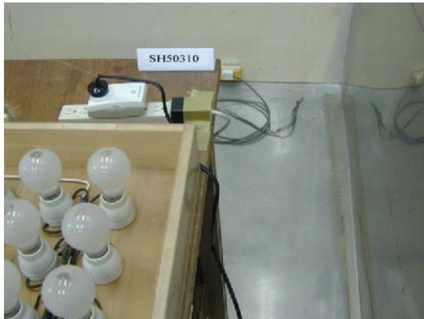
Photo 2: Conducted Test Set-up (rear)
