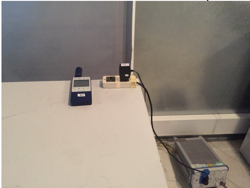
Measurement of Conducted Emission Test Set Up
