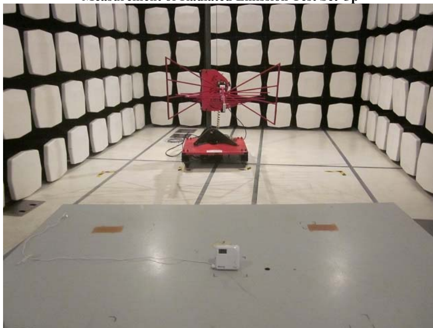
Measurement of Radiated Emission Test Set Up
