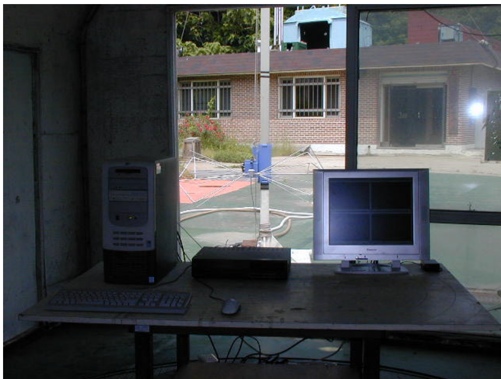
RADIATED EMISSION SETUP PHOTOGRAPH - FRONT VIEW ( 30 - 300 MHz )
