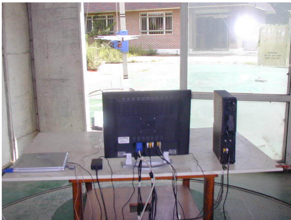
RADIATED EMISSION SETUP PHOTOGRAPH - REAR VIEW ( 300 - 1000 MHz )
