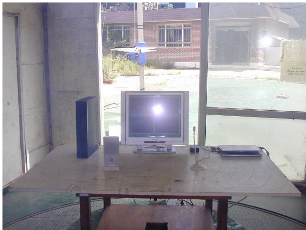
RADIATED EMISSION SETUP PHOTOGRAPH - FRONT VIEW ( 300- 1000 MHz )
