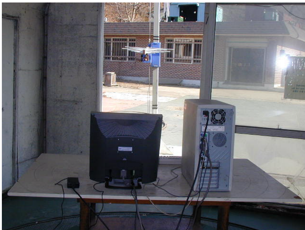
RADIATED EMISSION SETUP PHOTOGRAPH - REAR VIEW ( 300 - 1000 MHz )
