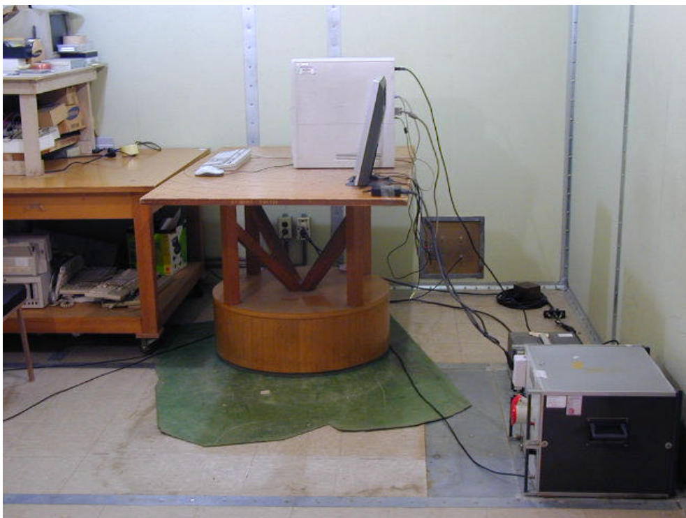
LINE CONDUCTED SETUP PHOTOGRAPH - REAR VIEW
