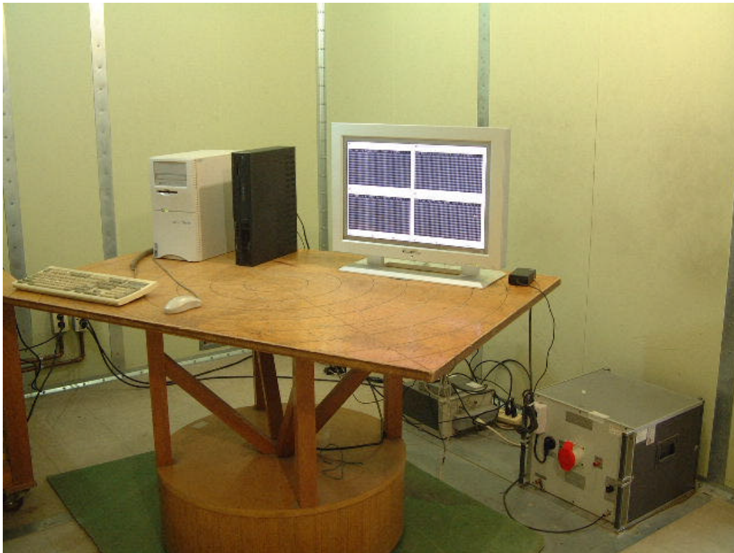
LINE CONDUCTED SETUP PHOTOGRAPH - FRONT VIEW
