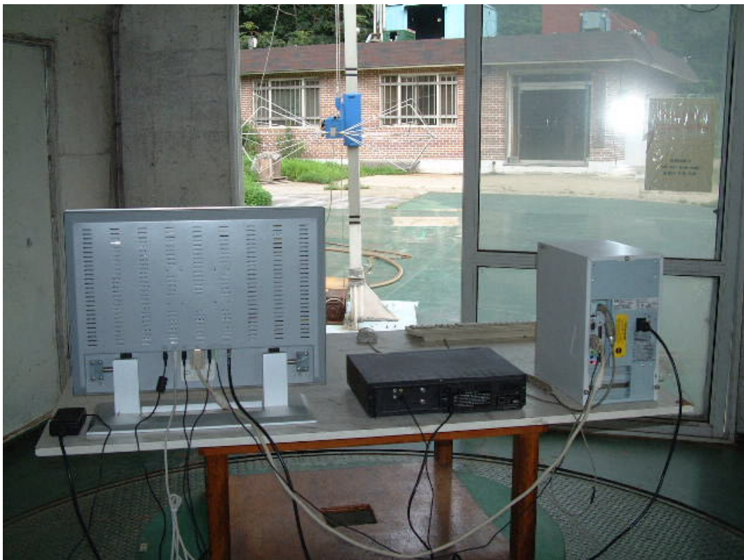
RADIATED EMISSION SETUP PHOTOGRAPH - REAR VIEW ( 30 - 300 MHz )
