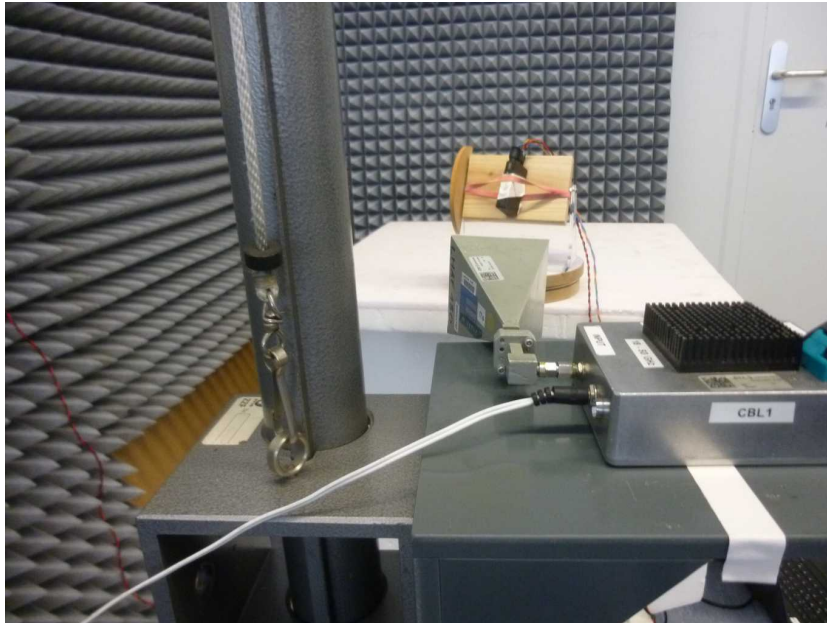
Photo 7: UWB 18 GHz to 40 GHz test setup
