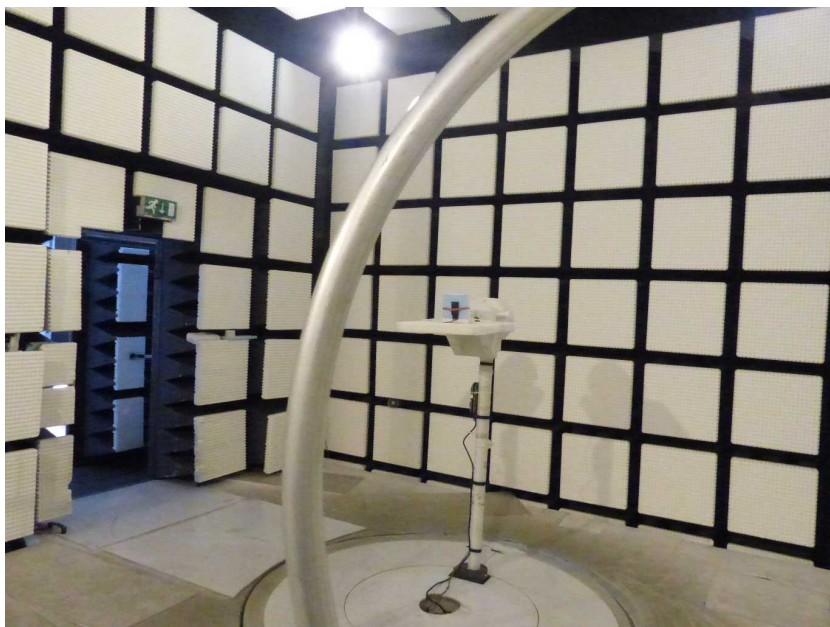
Photo 6: EUT at the fully anechoic chamber
